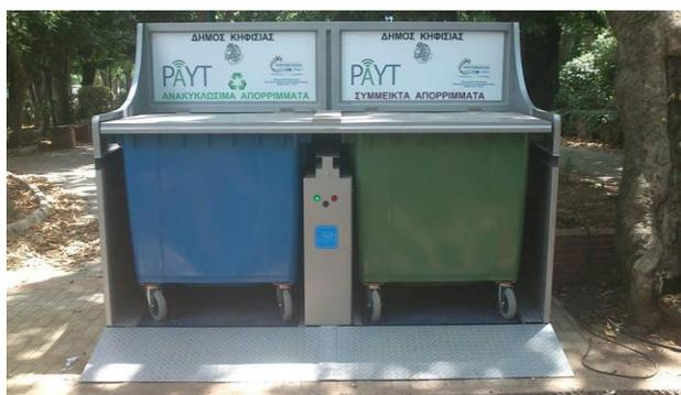
The developed dual-bin system with user identification and integrated bin weighing.
