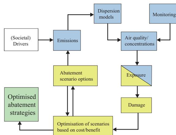
Functional structure of modules in an integrated Air Quality Management system
