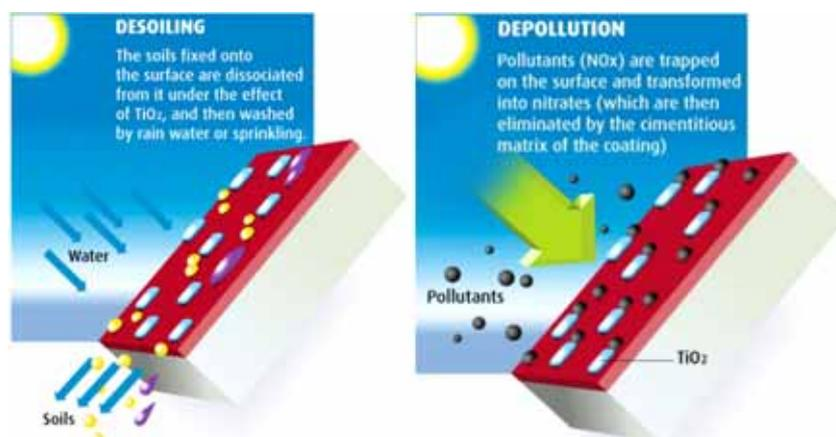
*The de-soiling and de-polluting abilities of the PICADA materials are due to the introduction of suitable amounts of titanium dioxide.*
