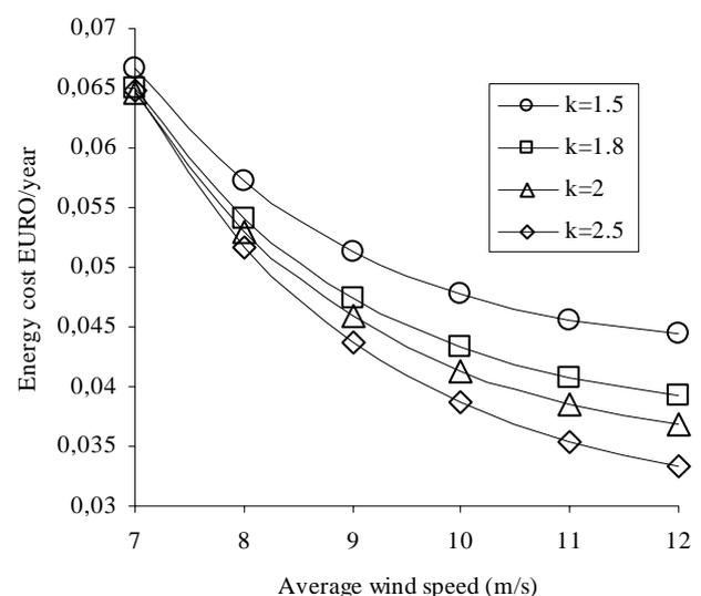
Energy production costs of a Bonus 300/33.4 Mk III wind turbine as function of average wind speed and shape factor,  $r=7\%$  and  $n=15$  years
